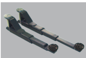
Support arms, telescopic and double telescopic ECON III 3.0 (option)
