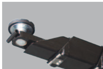
Support arm extensions running on roller bearings ECON III 5.0
